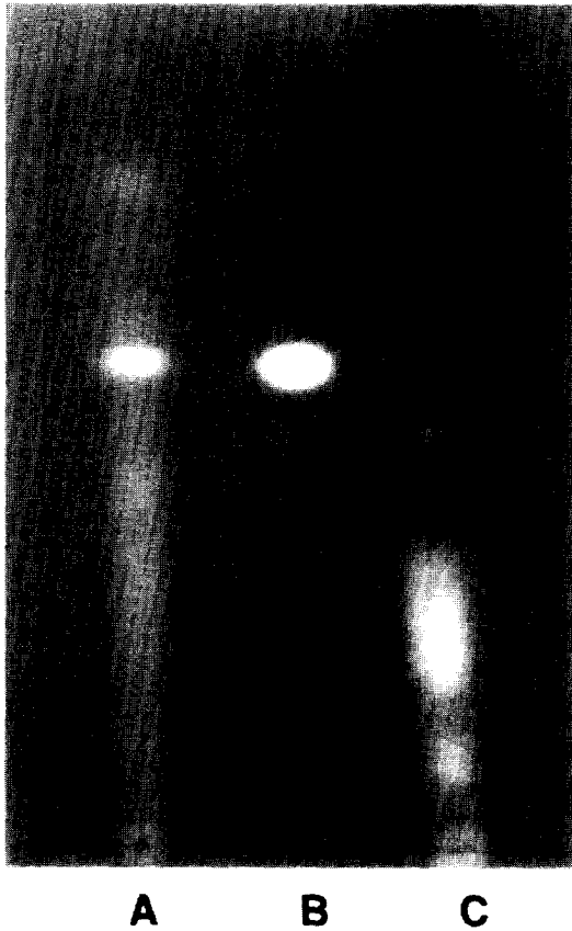
Fig. 1. TLC bands obtained for (A) a solution treated with activated charcoal after extraction from dung spiked with 100 ng ivermectin, (B) a reference solution of 100 ng ivermectin and (C) a solution not treated with activated charcoal after extraction from dung spiked with 100 ng ivermectin. All samples were derivatized.
